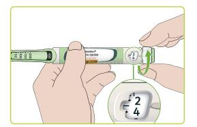
Max SoloStar: Select 4 units by turning the dose selector until the dose pointer is at 4.
